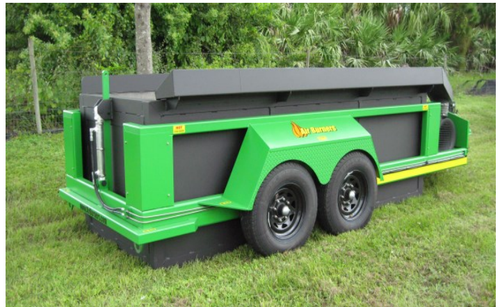
T24 BurnBoss - Firebox Lowered to Ground
