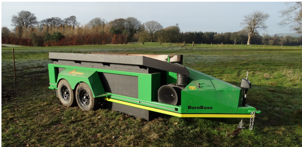
T24 BurnBoss Trailer Mounted FireBox (Firebox DOWN in Operational Mode)
