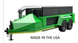
**General:** The T24 is a towable self-contained, completely assembled above ground Air Curtain Burner for mobile applications. It has been fitted with a refractory lined burn-container that is raised and lowered by a hydraulic lift system. Designed for the environmentally sound high temperature reduction of clean wood waste in forestry and agriculture in compliance with the requirements of U.S. EPA 40CFR60, the T24 is also used for disaster recovery and DHS/FEMA contingencies.
