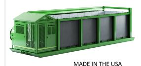
**General:** A self-contained above ground Air Curtain Burner (FireBox or air curtain incinerator) with a refractory lined burn-container for portable and stationary applications. Designed for the environmentally friendly high temperature reduction of clean wood waste in forestry, agriculture, land clearing, at landfills, transfer stations, etc. in compliance with the requirements of US EPA 40CFR60.
