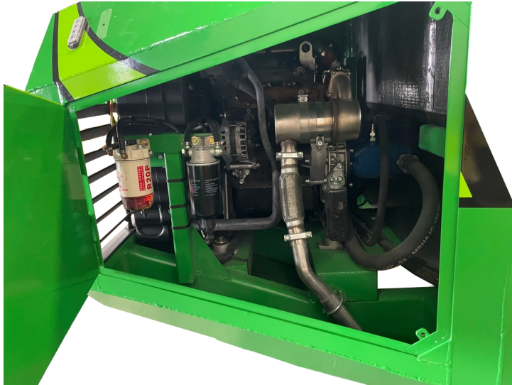
Left Access Door to HATZ Diesel Engine
