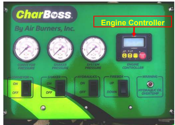
Control Panel with Toggle Switches & Gauges (See Page 13 for Enlarged Image)
