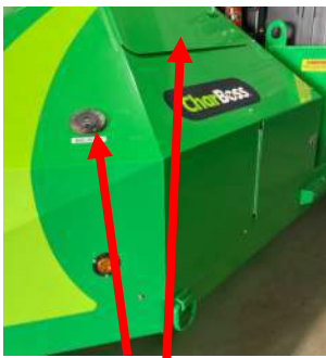
Upper Service Access & Diesel Fuel Fill
