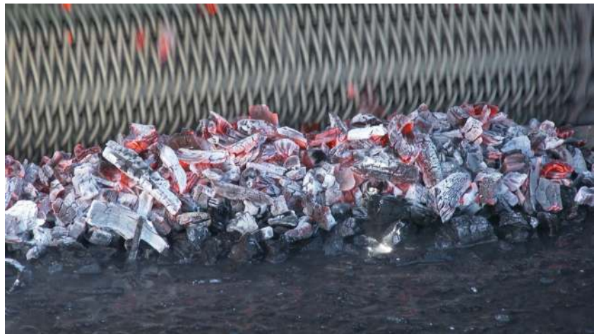
Char Exiting Conveyor Before Quenching
