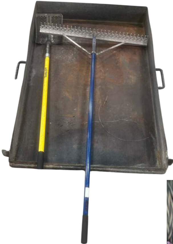
Quenching Bin/Biochar Collection Tray with Implements
