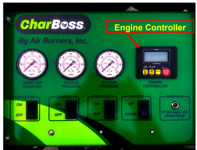
Control Panel with Toggle Switches & Gauges (See Page 13 for Enlarged Image)
