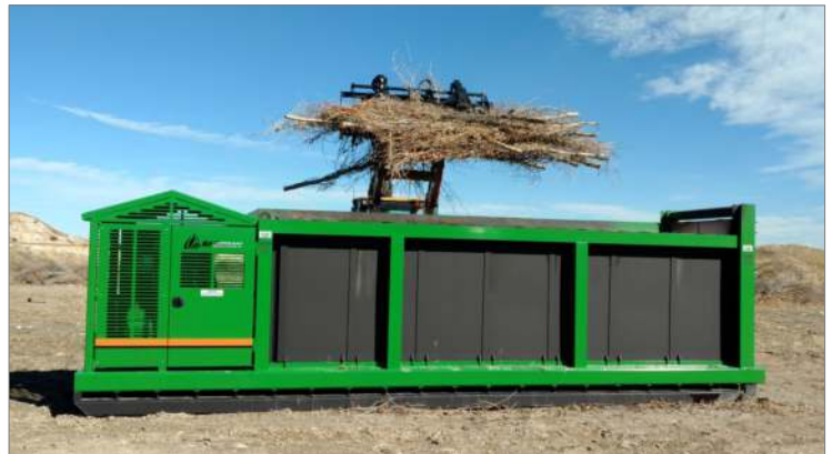
S119R Roll-Off FireBox Loading Over Manifold
