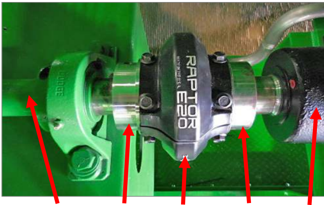
FAN SHAFT HUB ELEMENT HUB FLUID CLUTCH
