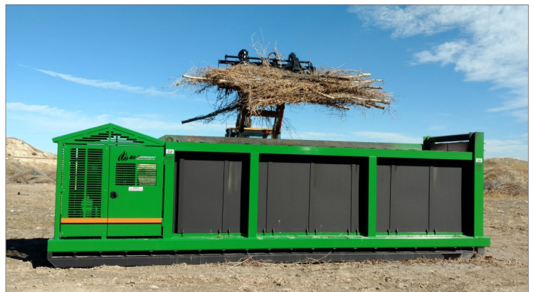
S119R Roll-Off FireBox Loading Over Manifold
