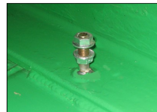
Grounding Stud (Location may vary)
