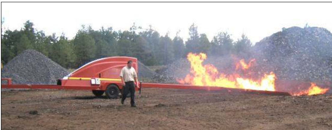
LIGHT-OFF , Changing from Darker Wispy Smoke of Diesel to White Smoke from Burning Wood.
