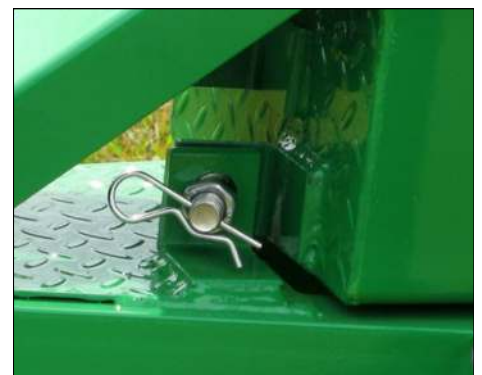
Safety Bolt Securing Retracted Manifold Assembly
