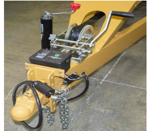
Ball Hitch Adapter (Pintle Hitch Optional), Safety Chains, Pigtail, Winch, Break-away Unit & Front Jack Stand
