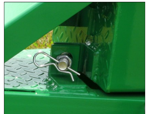
Safety Bolt Securing Retracted Manifold Assembly
