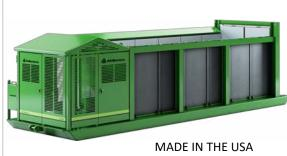
**General:** A self-contained above ground Air Curtain Burner (FireBox or air curtain incinerator) with a refractory lined burn-container for portable and stationary applications. Designed for the environmentally friendly high temperature reduction of clean wood waste in forestry, agriculture, land clearing, at landfills, transfer stations, etc. in compliance with the requirements of US EPA 40CFR60.
