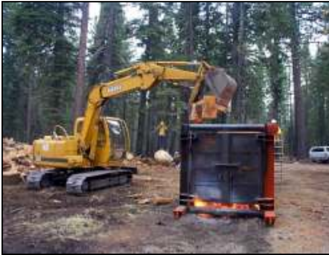
Figure 4—Loading fuel into ACD (full operation).
