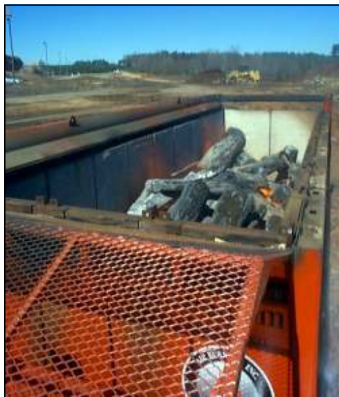
Figure 1—ACD in full operation (no visible smoke).
