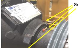
Grease at both sides of the engagement shaft and on top.
