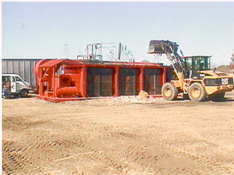
Figure No. 4 Whitton Technology, Inc. S-Series Air Curtain Destructor Operating at Full Capacity, No Visible Emissions
