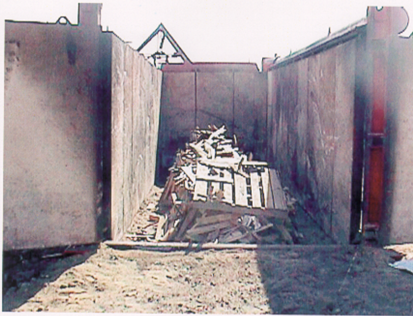
Figure No. 1 Whitton Technology, Inc. S-Series Air Curtain Destructor Refractory Lined Combustion Chamber
