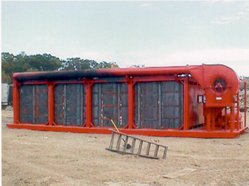
Figure No. 3 Whitton Technology, Inc. S-Series Air Curtain Destructor Blower and Air Manifold
