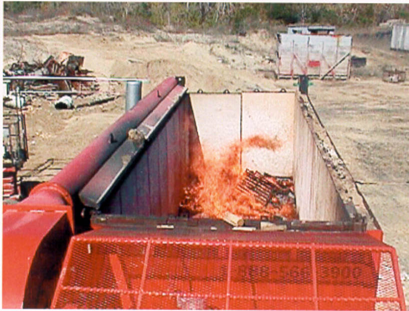
Figure No. 6 Whitton Technology, Inc. S-Series Air Curtain Destructor Operating at Full Capacity, No Visible Emissions
