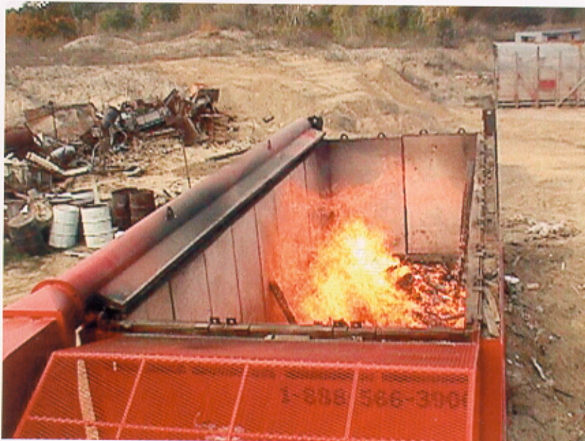
Figure No. 2 Whitton Technology, Inc. S-Series Air Curtain Destructor Initial Combustion, Air Manifold at Left
