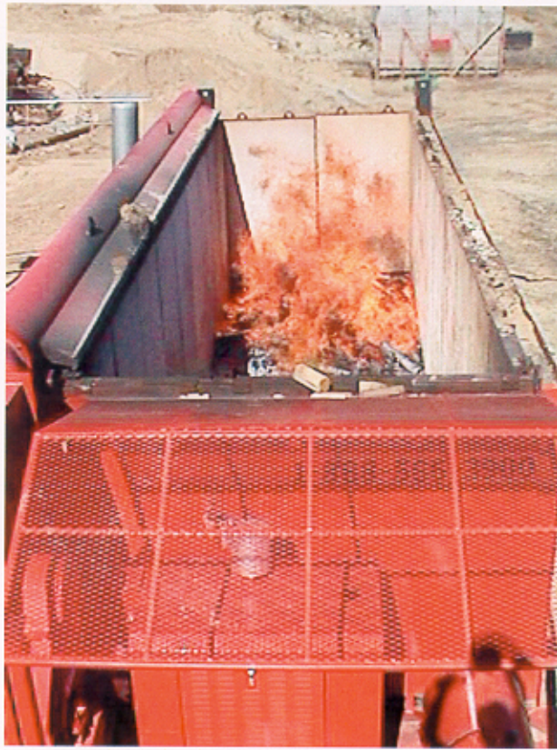
Figure No. 5 Whitton Technology, Inc. S-Series Air Curtain Destructor Operating at Full Capacity, No Visible Emissions
