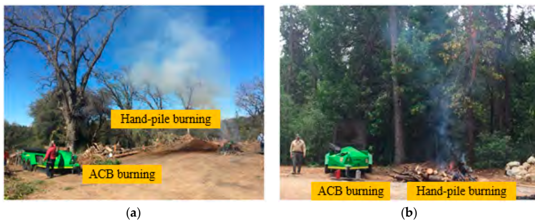
Figure 4. Comparison of the smoke occur from BurnBoss and hand-pile burning for the same types of forest residues; (a) Groveland and (b) Volcano, California. BurnBoss burnings shows little smoke and air pollutants, compared to hand-pile burnings.
