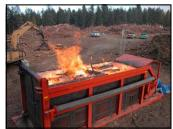
In October of 2002, scientists from the Missoula Fire Sciences Laboratory (FiSL) teamed with engineers from the San Dimas Technology and Development Center (SCTDC) to evaluate the performance of an air curtain incinerator. A model 217, with a capacity of 6 tons per hour, was provided by the manufacturer. Other air curtain burners, with through-puts ranging from 1 to 15 tons per hour, are available from Air Burners LLC. For more information contact them at www.airburners.com
