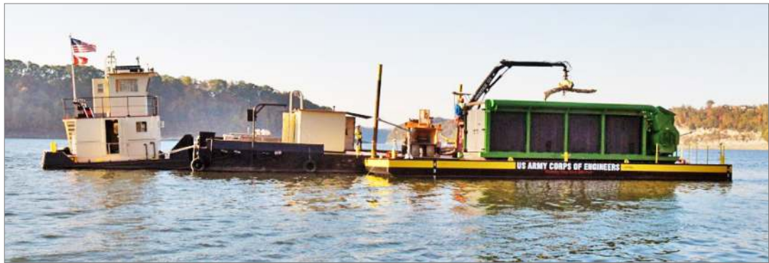
"Pride of the Cumberland": Feeder & Loading Barge (left) and Debris Eliminating FireBox Barge
