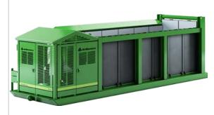
**General:** A self-contained, completely assembled above ground Air Curtain Burner (air curtain incinerator or FireBox) with a refractory lined burn-container for stationary applications. Designed for the high temperature reduction of wood waste in forestry, agriculture, land clearing, at landfills, transfer stations and other waste streams in compliance with the requirements of US EPA 40CFR60.
