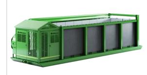
**General:** A self-contained, completely assembled above ground Air Curtain Burner (air curtain incinerator or FireBox) with a refractory lined burn-container for stationary and mobile applications. Designed for the high temperature reduction of wood waste in forestry, agriculture, land clearing, at landfills, transfer stations and other waste streams in compliance with the requirements of US EPA 40CFR60.
