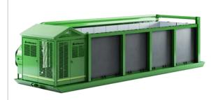
General: A self-contained, completely assembled above ground Air Curtain Burner (air curtain incinerator or FireBox) with a refractory lined burn-container for stationary applications. Designed for the high temperature reduction of wood waste in forestry, agriculture, land clearing, at landfills, transfer stations and other waste streams in compliance with the requirements of US EPA 40CFR60.
