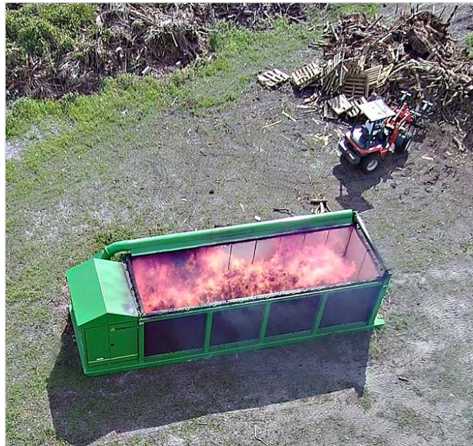
Air Burners Model S-327 in Full Operation at a Wood Waste Collection Site
