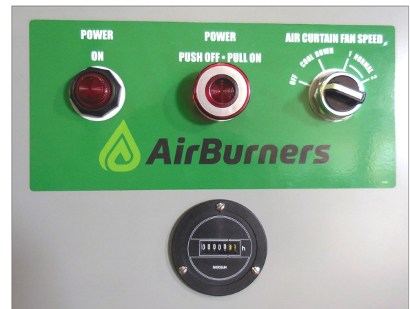
Control Switches (Main Power Button in Center), Indicator Lights & Hour Meter
