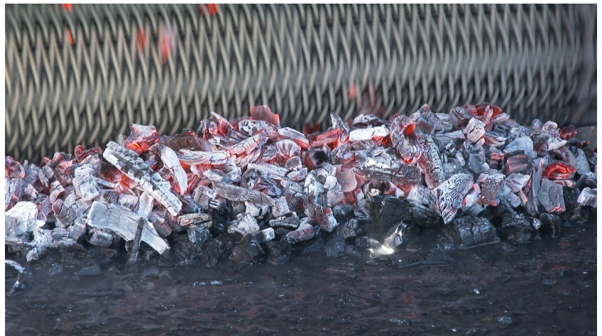
Char Exiting Conveyor Before Quenching
