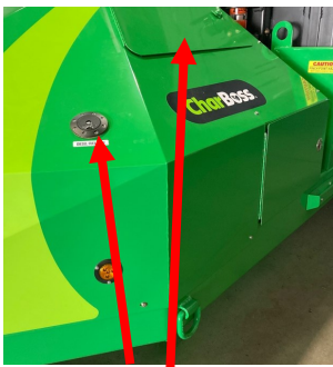
Upper Service Access & Diesel Fuel Fill
