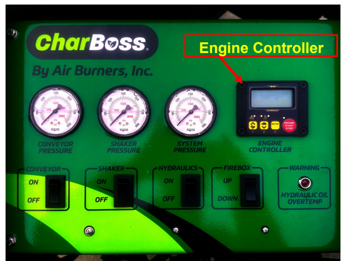
Control Panel with Toggle Switches & Gauges (See Page 13 for Enlarged Image)
