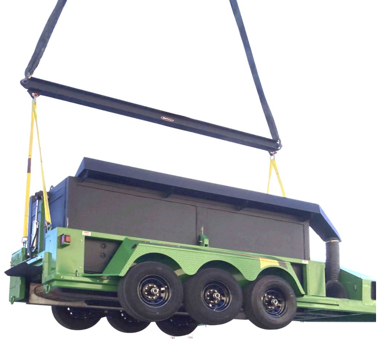
Rear Lifting Points and T26 Spreader Bar
