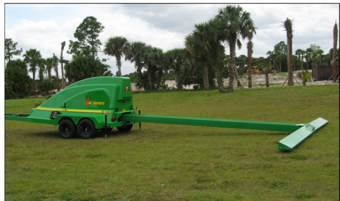
T300 Carrier Pipe Fully Extended and Manifold on the Ground
