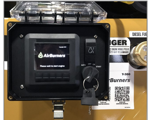
Electronic Control Panel (Lockable Cover Open)
