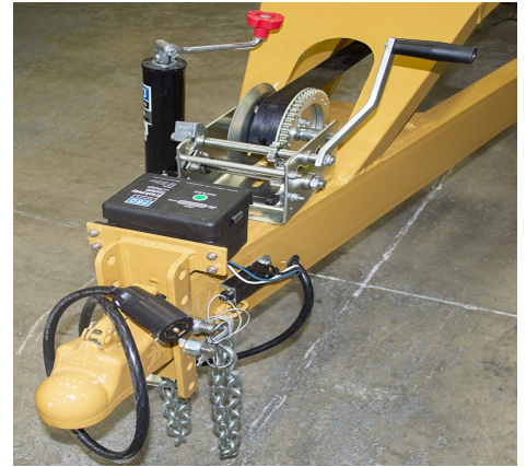
Ball Hitch Adapter (Pintle Hitch Optional), Safety Chains, Pigtail, Winch, Break-away Unit & Front Jack Stand
