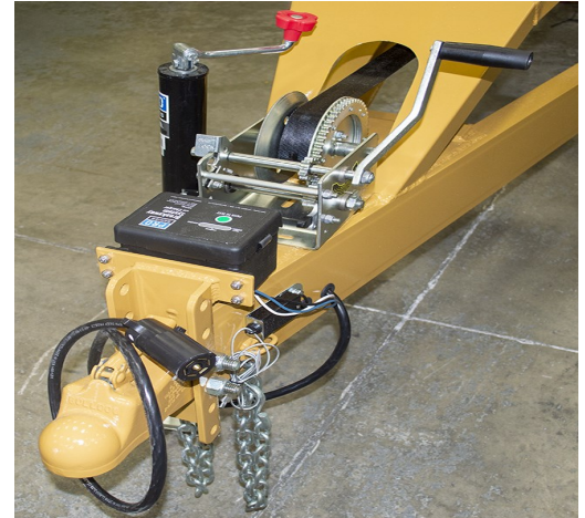
Carrier Pipe, Winch, Jack Stand, Safety Chains, Ball Hitch Receiver, Break-away System and Pigtail with 7-Blade RV Plug
