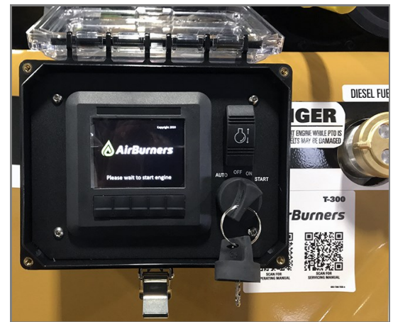
Electronic Control Panel (Lockable Cover Open)
