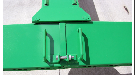
Locking Bolt at Center of the Manifold
