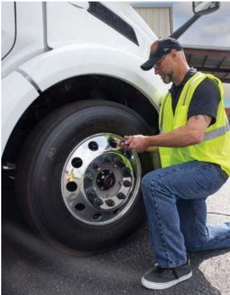
The driver checks the tire monitoring sensor attached to the valve stem. Photos courtesy of Bridgestone.
