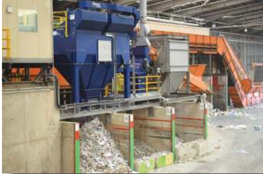
Glass and SRF material separation with Impact's ZAC (Zigzag Air Classifier).
