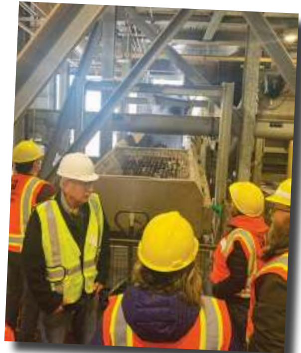
After exiting the Juno Clave, the material goes into a wet separation unit that uses Georgia-Pacific's extensive knowledge of paper fiber cleaning to separate the paper fibers from the rest of the waste. This is what sets Juno apart from other waste and recovery technologies. Photos courtesy of Juno.
